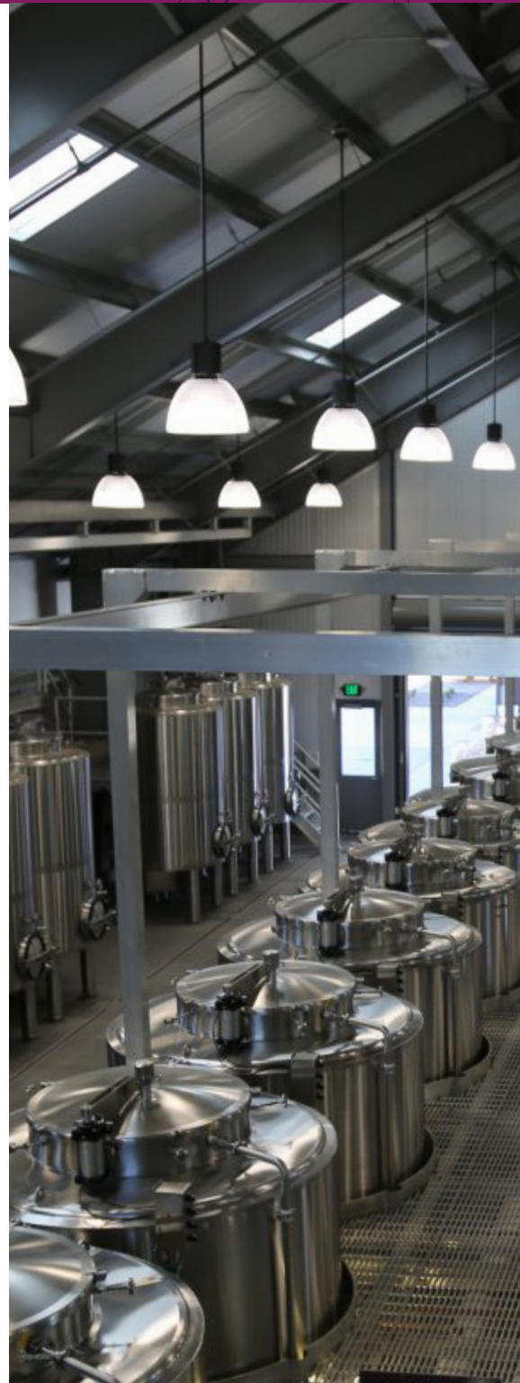
4-5 Ton Voltage Series Wine Tanks with AirLift Top Door; photo courtesy of Wheeler Farms Winery
