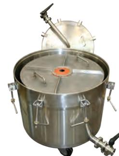
Internal Perforated Drain Screen
