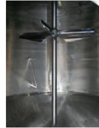
the cleaning cycle and is difficult to clean. The Sanifoil impeller design has eliminated impeller CIP shadows and comes standard on all our Yeast Brinks.
